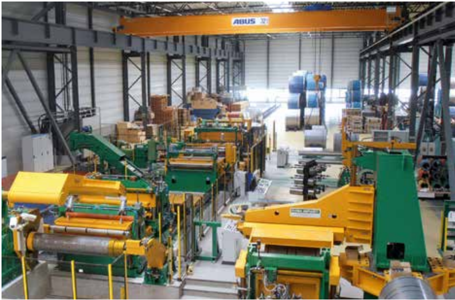
Guida slitting line: strips in thicknesses of up to 6 mm are possible.
