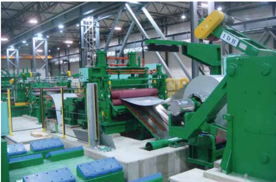
Hitachi cut-to-length line: continuous operation is guaranteed by two stack nest containers.
